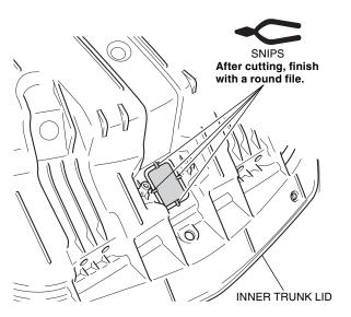
3. Install the trunk inner lamp as shown.
