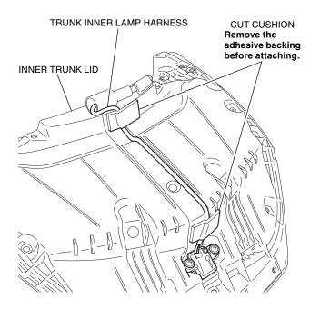
9. Install the inner trunk lid to the trunk lid as shown.
