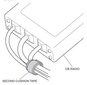
6. Attach the CB radio in the position shown.
