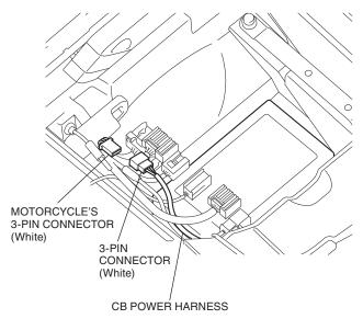
9. Connect the CB antenna harness as shown.
