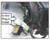
Remove the clip and **TWIST the 4-pin connector around** to plug the **pathBlazer** in-line. The female socket can only go in one-way.
