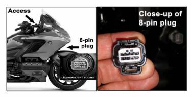
P115W-H3-GL8 has matching 8-pin plug and socket for the LED headlights.
