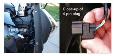
P115W-H3-WK4 has matching 4-pin plug and socket for the Valkyrie LED headlights.
